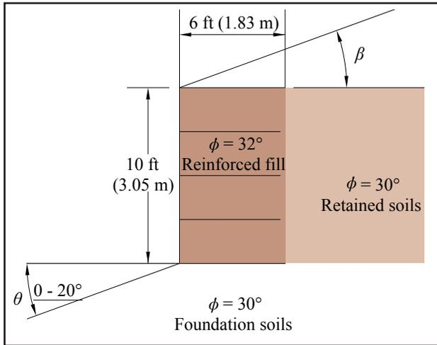
**Figure 3**—Typical Section for Figures 4 and 5
