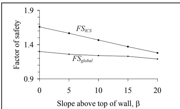
**Figure 5**—Effect of Slope Above Top of Wall
