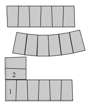
Placing the units in an alternating pattern creates a straight section.
